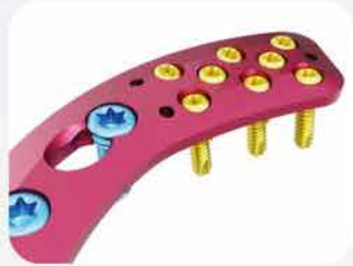
The elongated Combi hole in the neck and shaft enables plate adjustment and provides options for locking or compression.
